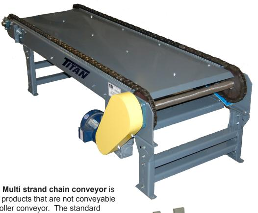
The Model 680 Multi strand chain conveyor is used to convey products that are not conveyable on a standard roller conveyor. The standard chain is C2060 double pitch with a load capacity of 2,400 lbs. An optional C2080 double pitch chain can be used for loads up to 4,000 lbs. Optional low profile side mounted drive and additional strands of chain can be added to increase load capacities.
