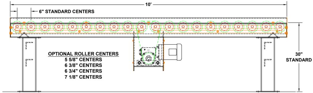
STANDARD 10' LG. CONVEYOR SECTION W/#60 CHAIN DRIVE
