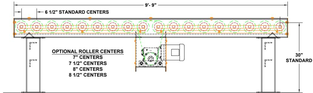
STANDARD 9'-9" LG. CONVEYOR SECTION W/#80 CHAIN DRIVE
