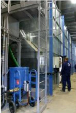
Beginning at the blast machine the pressure and abrasive content is set to the required limits. Once the operator has closed the dead-mans handle, abrasive is propelled under pressure through a high quality 12 bar blast hose of 1.25" bore and in-turn the blast nozzle. This is only possible provided all safety interlocks are closed on doors, etc.
