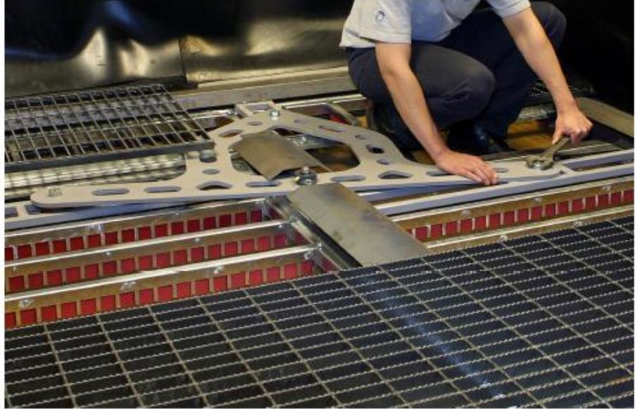
Several corridors run the length of the facility deploying abrasive into a transversal corridor running at right angles to the longitudinal corridors. In this case a pit, with recovery floor, is facilitated by dropping the transversal below it by 130mm.
